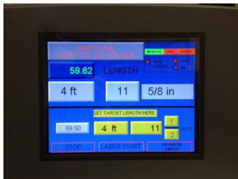
Cut-off system monitor controls cut length and adjusts feed rate as target approaches desired length.
